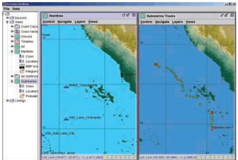
Figure 3. CoAX Binni 2002 – Submarine contacts from the underwater sensor grid are delivered to QinetiQ's Decision Desktop tool via the dynamic agent infrastructure. The rightmost panel shows that the commander has chosen to display them according to their confidence level.
